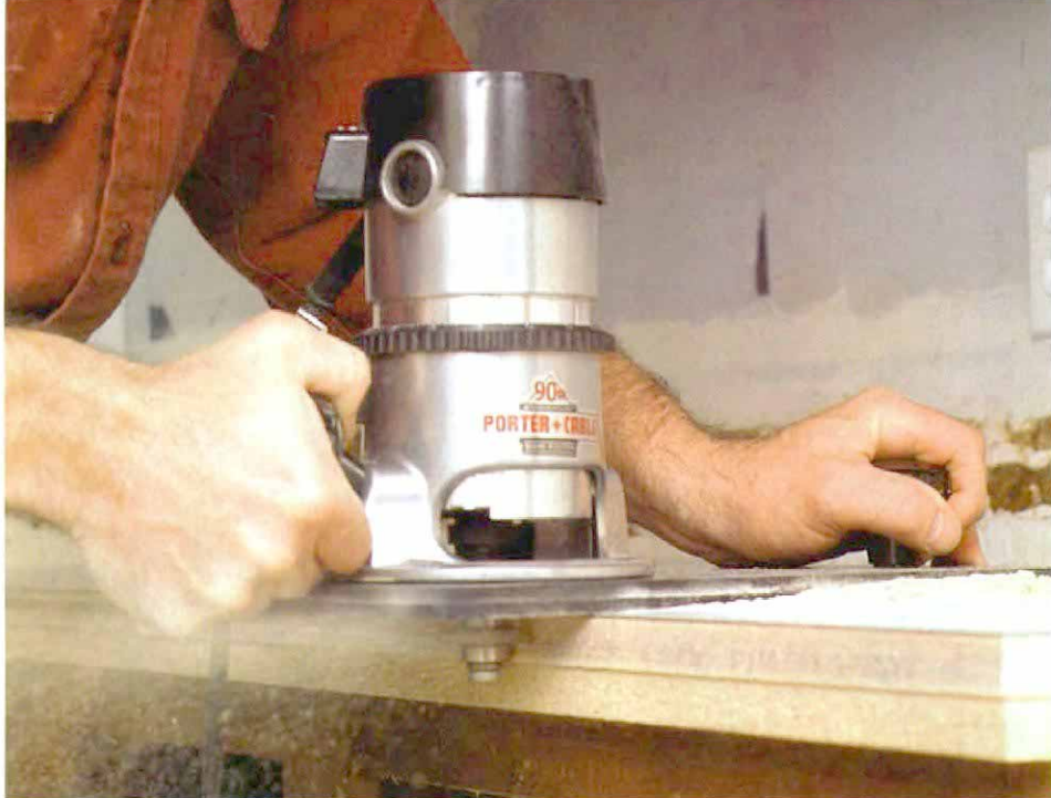
A 1/4-in. slotting bit grooves the top for tongued-back moldings. Careful location of the groove ensures that the top of the bevel molding will meet the top laminate perfectly.
