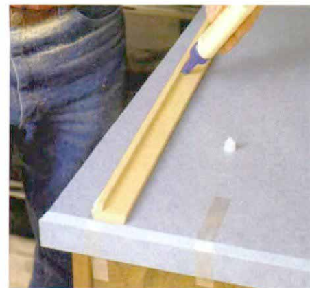
A small bead of glue on both sides of the tongue holds the molding in place. Too much glue can keep the molding from seating in the groove, resulting in an open joint.
